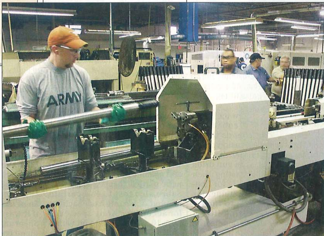
A machinist loads a .50-caliber barrel into the Sunnen HTB-2000 hone at Sabre Defence Industries, Nashville.
