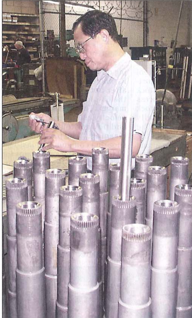
Stellite liners are individually OD ground to size, measured with a micrometer, and pressed into their mating, induction-heated barrels. A liner sticks out of a barrel awaiting press fitting.
