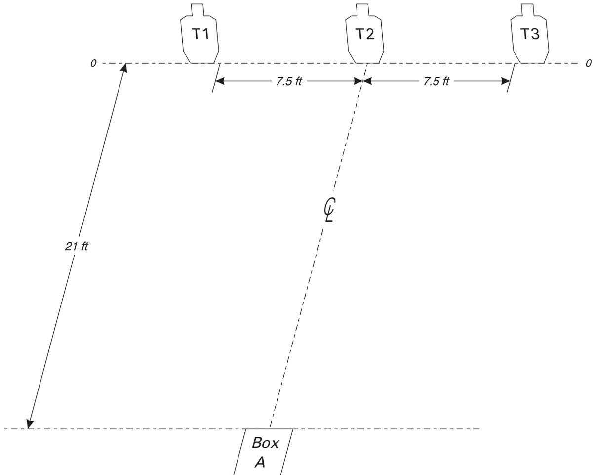
**SETUP NOTES:** Set paper targets to 5 feet high at shoulders. Box A is 3 feet by 3 feet. Angle T1 and T3 to face shooting box.
