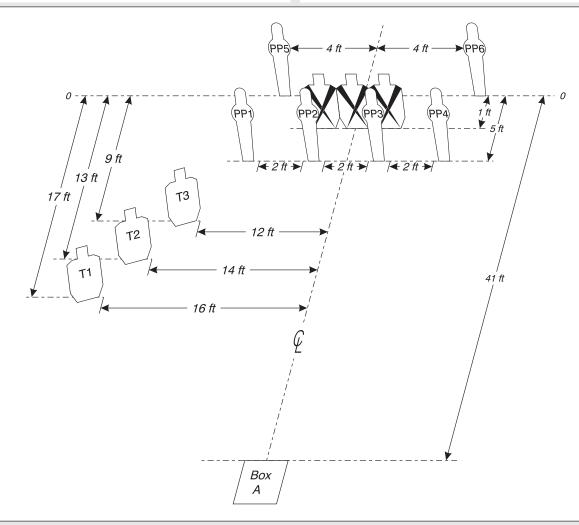
**SETUP NOTES:** Angle T1-T3 toward shooting Box A with right edge of each target placed at distances indicated. Box A is 3 feet by 3 feet. Set paper targets and no-shoots to 5 feet high at shoulders. No-shoots
