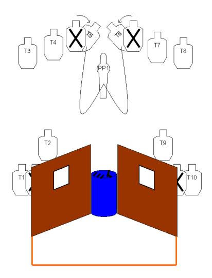
**SETUP NOTES**: Cant stages 3 & 4 into their respective corners by 5 to 10° to prevent shoot throughs from T10. T2-T9 are arrayed to avoid shoot throughs and splatter from PP1.
